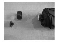
2. Push out the pin holding the retaining plug.
