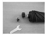
1. To remove the old canopy unscrew the metal tip and then the plastic nut at the top of the canopy.
